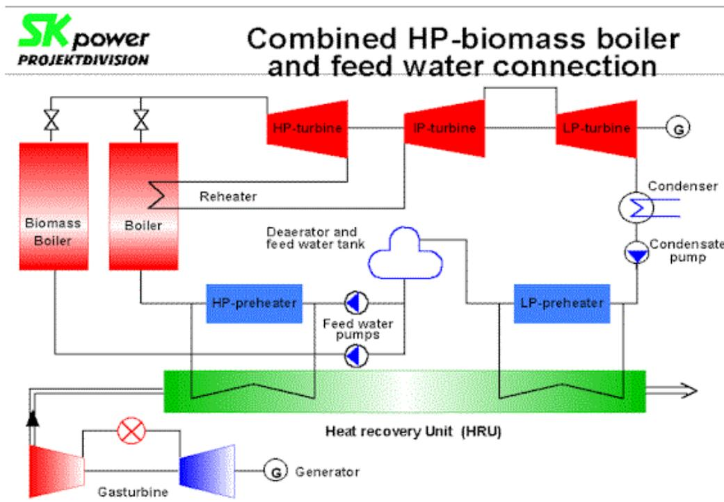
Figure 32 Configuration of the Avedøre 2 power plant<sup>32</sup>
