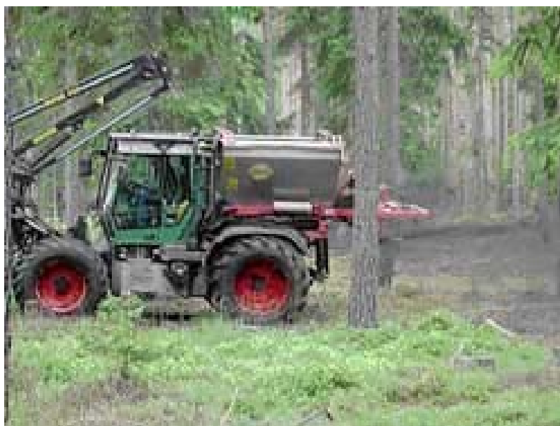
Figure 3. Ash spreading with tractor (Swedish National Board of Forestry).
